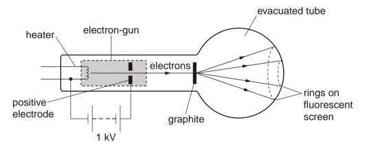
The electrons are accelerated to high speeds by the electron-gun. These high speed electrons pass through a thin layer of graphite (carbon atoms) and emerge to produce rings on the fluorescent screen.
